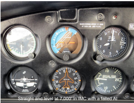
Straight and level at 7,000' in IMC with a failed AI
