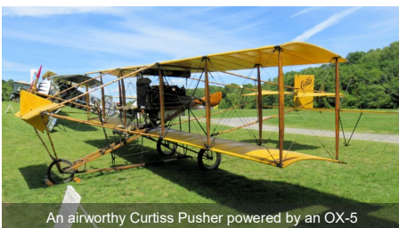
An airworthy Curtiss Pusher powered by an OX-5
