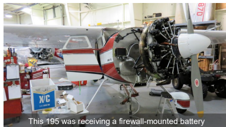
This 195 was receiving a firewall-mounted battery
