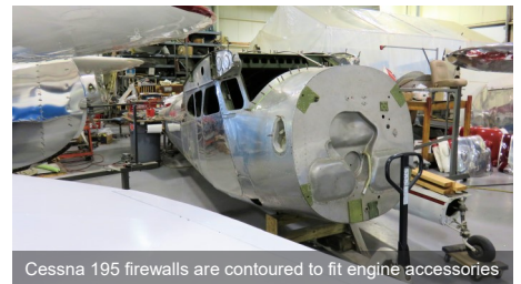
Cessna 195 firewalls are contoured to fit engine accessories
