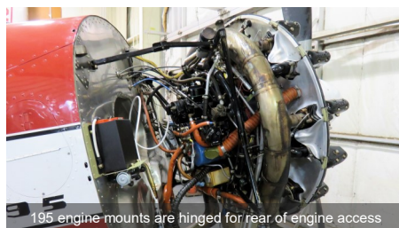
195 engine mounts are hinged for rear of engine access
