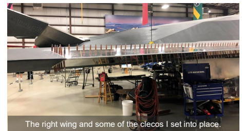
The right wing and some of the clecos I set into place.
