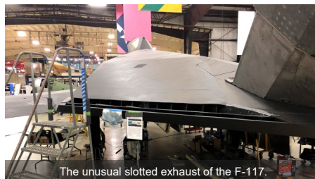
The unusual slotted exhaust of the F-117.
