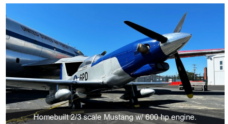
Homebuilt 2/3 scale Mustang w/ 600 hp engine.
